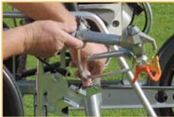
No-tools gun removal for easy spraying of numbers, logos and other field markings.
